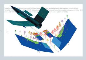
aeroelastic capabilities for stress, load, aerodynamic and control system analysis and design using a common finite element representation.
