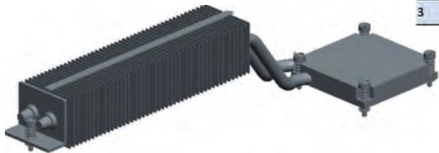
Figure 3. Detail of Heat Pipe Design for IC
