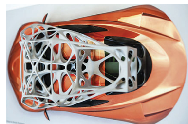
Figure 9. Aquilo concept car design in PTC Creo with external aerodynamics pressure predictions from FloEFD Simulations
