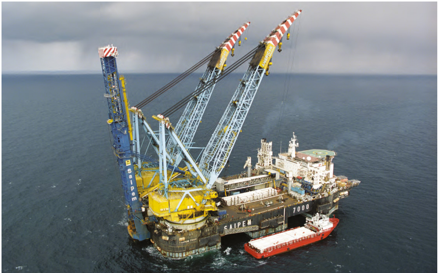
Figure 1. The Saipem 7000: The world's second largest Semi-Submersible Crane Vessel (SSCV)
