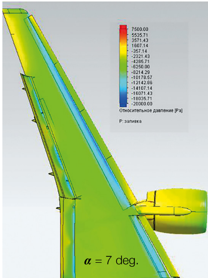
Figure 4. Computation Results: \Delta P on Wing Surface
