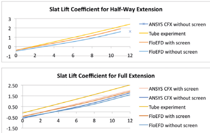
Figure 7. Results Comparison: Slat Lift Coefficient
