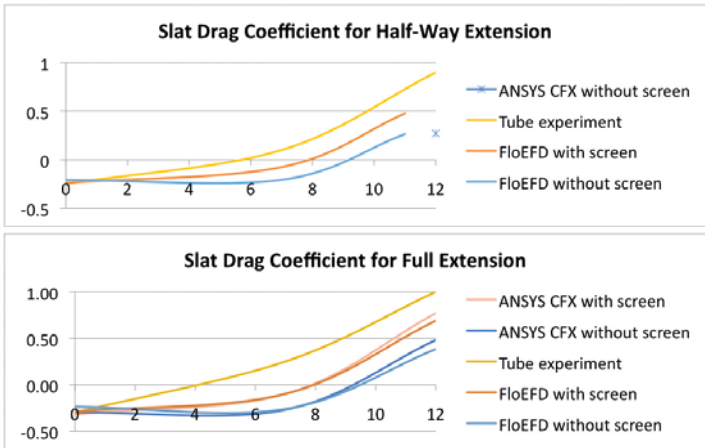
Figure 6. Results Comparison: Slat Drag Coefficient
