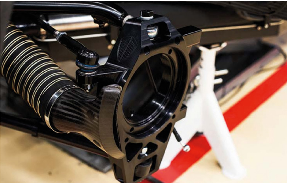
Figure 3. Brake cooling duct mounted on a Koenigsegg Regera upright (the baseline design). (Klingelhofer, 2013, Ref 3)
