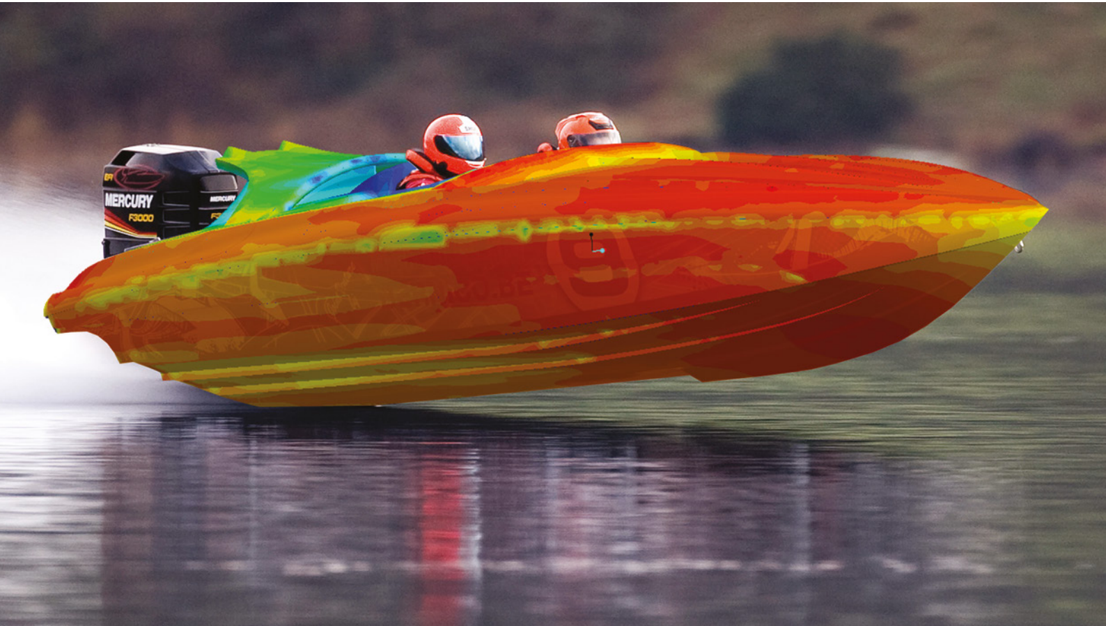
Figure 4. Record Breaking F2 Bernico Boat on Coniston Water in November 2009 with superimposed hull pressure contours from FloEFD simulation prediction
