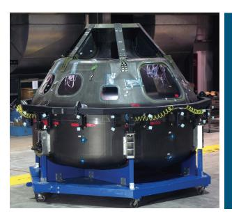
The composite crew module is shown during the assembly splice operation at ATK in luka, Mississippi, USA, prior to the installation of graphite epoxy doublers. The use of Fibersim helped NASA capitalize on the potential of composite materials by reducing risk, design and manufacturing costs as well as complexity and cycle times. The software has proven in production to increase engineering productivity and reduce development time, material waste, design revisions and tooling costs.
