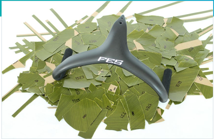
The handlebar SL11 for a sprint bicycle, representing 136 parts, is the result of component optimization using NX Nastran. Copyright: FES.
