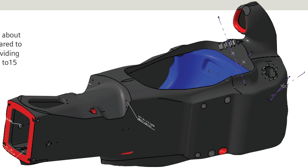
A Monocoque chassis made of carbon fiber is one of the most difficult composite parts to design and manufacture for Formula One race cars due to the complexity of the shape and layup. Shown is a solid model of the final Monocoque chassis, which was designed and manufactured using Fibersim.
