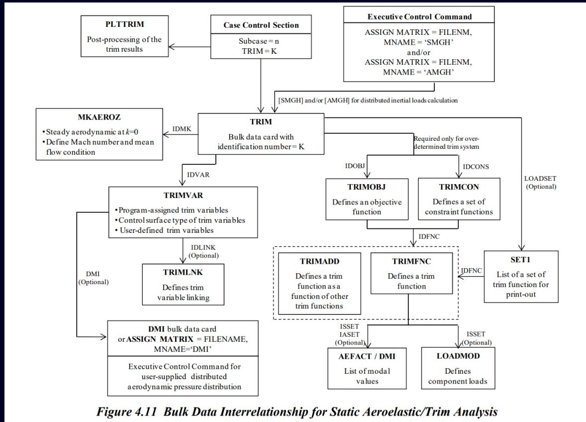
Figure 4.11 Bulk Data Interrelationship for Static Aeroelastic/Trim Analysis
