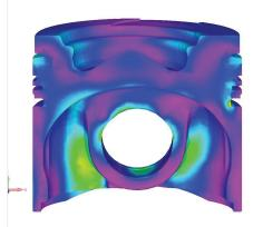
"Using the data obtained with Femap, we can determine whether or not the piston's initial design requires any major changes. If major changes aren't necessary, the next step is to create the first castings and to carry out the subsequent mechanical machining operations to construct the piston to be tested."
